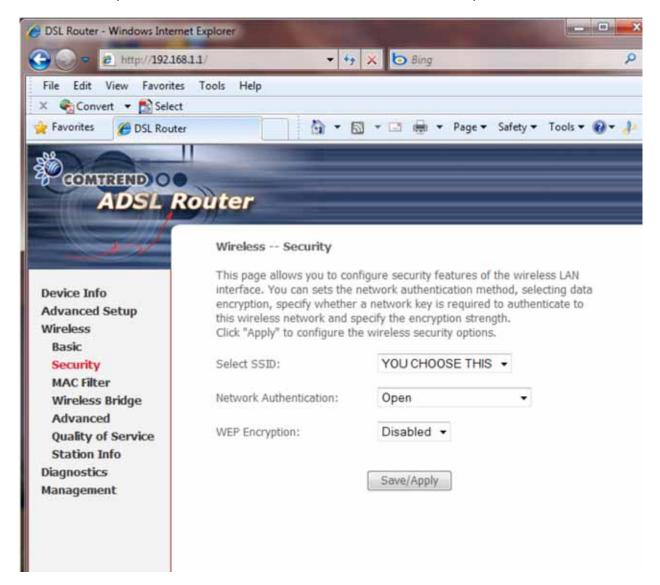
Make sure the Selected SSID is set the SSID that you have just created.
